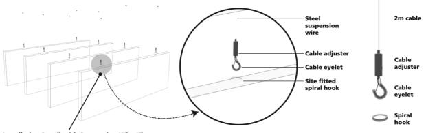
Installation Detail with Suspension Wire Kit
